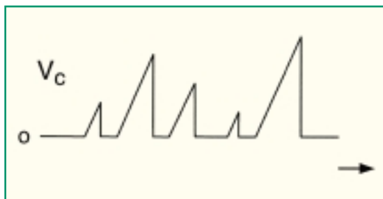
Fig. 14b. V_C = 0 when SW closed, V_C > 0 when SW open
